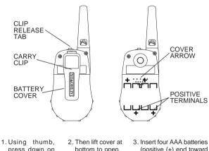
bottom to open (positive (+) end toward the top begining at left Remove cover side and alternating positive terminals as
