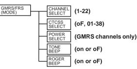
NOTE: To differentiate between operating modes, look for HI or LO indication below the battery power level indicator when in GMRS mode. Refer to the appropriate section of this manual for de-tailed operating instructions for each mode. Channels 1 through 7 are shared GMRS/FRS. Channels 8 through 14 are FRS only, and channels 15 through 22 are GMRS only
